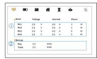
① Display the working parameters of the four channels of PV (PV1, PV2, PV3, PV4), including real-time voltage, current, and power. (PV input type can be set in the settings). ② Display the cumulative charging capacity of the PV, including daily and total accumulated energy.
