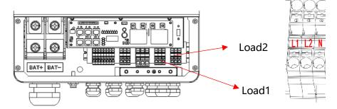
Inside the inverter, load2 is connected to load1 through a relay, and the relay disconnect when the SOC of battery is lower than set value. At that time, the load2 is powered off and load1 is still powered on. (The total power of Load1 plus Load2 should not more than the rated BACK-UP power when GRID is off)
