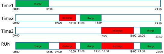
3) If you want to set a continuous charging time from the first night to the next morning. For example, you want to charge the battery from the first day 21:00pm to the next day 5:00am, divide this time period into two time periods ( $21:00\sim23:59$ ,  $00:00\sim05:00$ ), and select two charging time periods from Time1, Time2 and Time3 and set them.
