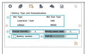
① Set Battery Type and Battery Communication method.
