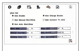
As shown in the picture on the left, select Gen Enable, Gen auto and Gen charge enable. Set generator on, off SOC or voltage, charging current, generator power, stop cooling time, maximum running time.
