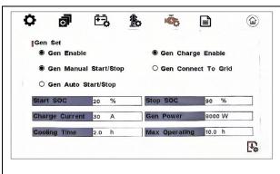
As shown in the picture on the left, select Gen Enable, Gen Manual and Gen charge enable. charging current, generator power, stop cooling time, maximum running time.
