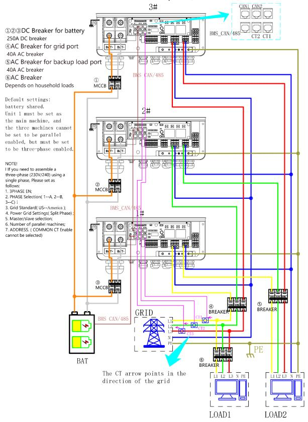
Multiple inverters can be installed together to deliver more power. When AC loads are present, all units effectively share the load.
