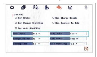
**Start Volt:** Generator in automatic mode. When the volt of battery is lower than the setpoint, the Generator dry contact is turn-on and the connected Generator will be started.
