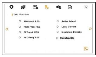
When the grid voltage is abnormal, the charging power will be limited, and the function will be enabled if required by the national grid standards.
