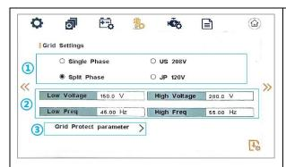
①Inverter use Split Phase, default option is Split Phase.(JP 120V is the reserved standard) ②**Low Voltage**: The input value of Grid low voltage. It is valid when grid mode selected custom.
