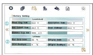
①Settings required when using lead-acid batteries
