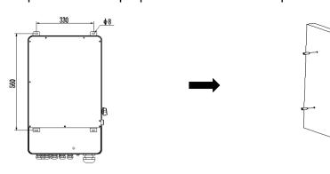
**Step 2**: Lift the inverter and align the hole of the inverter with the expansion bolt, Fix the inverter on the wall.
