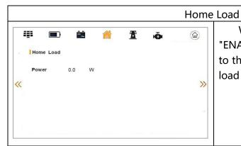
When set Home load EN to "ENABLE", if you have a load connected to the mains port, you can see its Home load power.
